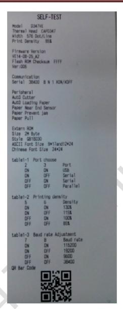
5) According to the self-test page, set the DIP switch position, accomplish the corresponding function requirements.
