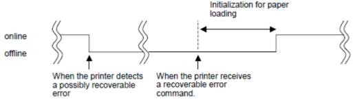
When the printer detects a possibly recoverable error, the printer goes offline.
