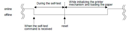
The printer goes offline during the self-test. When the self-test is ended, the printer is reset automatically.
