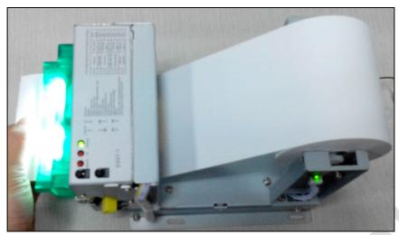
4. With the hand to block out of the paper, paper printers automatically stop, LED lights on, the paper feed smoothly, LED lights off, and then continue to print.
